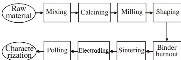
**Fig.4 :** Flowchart for the processing of ferroelectric ceramics
