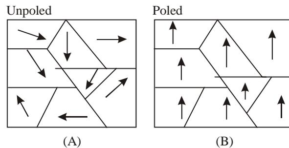
**Fig.5 :** Schematic of the poling process in piezoelectric ceramics : (a) In the absence of electric field the domains have random orientation of polarization; (b) the polarization within the domains aligns in the direction of the applied field.
