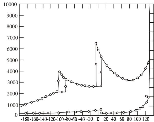
**Fig.3 :** Variation of dielectric constants (a and c axis) with temperature for  $BaTiO_3$ .
