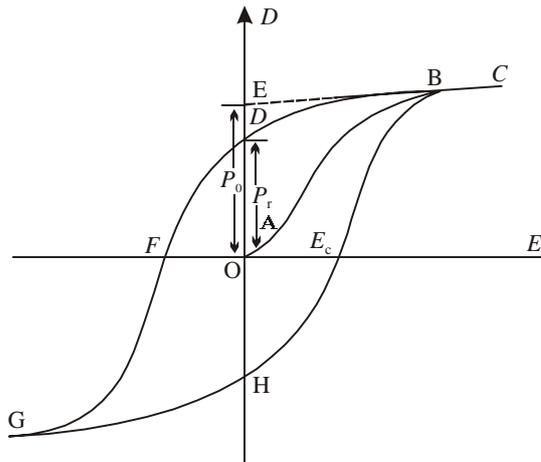
**Fig.2 :** A Polarization vs. Electric Field (P-E) hysteresis loop for a typical ferroelectric crystal
