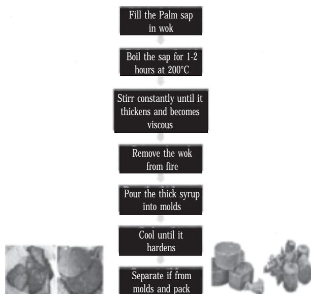
**Fig. 3 : Process Flow chart for manufacturing of Palm Jaggery**
