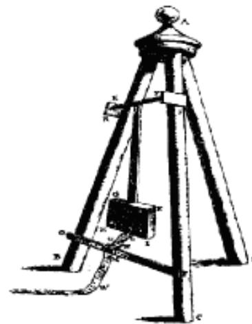
Fig. 1 Robins' Ballistic Pendulum as sketched in "The New principles of Gunnery"
