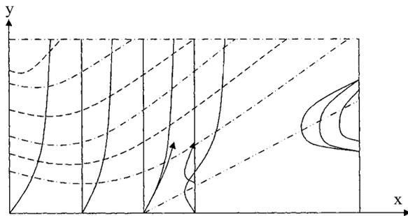
Figure 2 : Boundary Layer Separation
