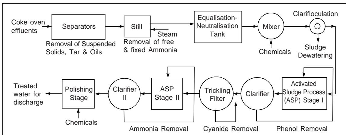
Fig. 1 : Process flow diagram for coke oven effluent treatment
